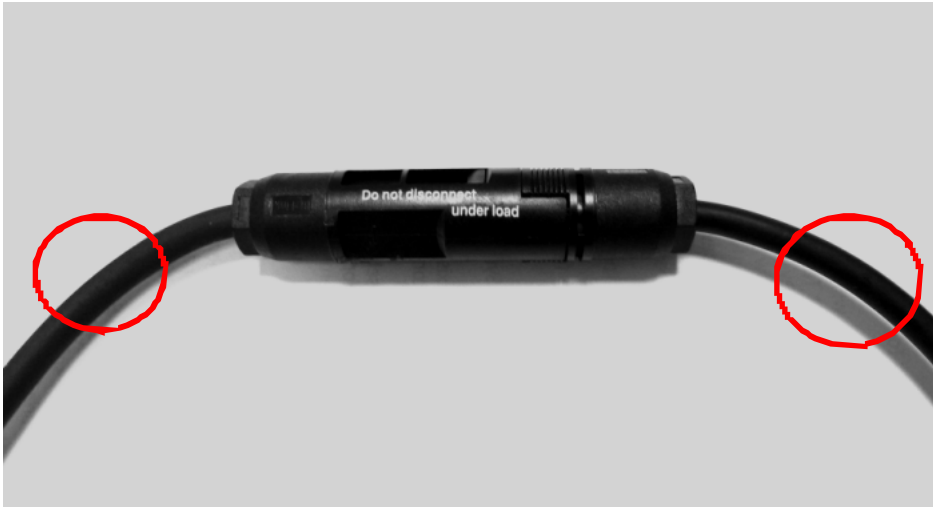
Correct Cable Routing
